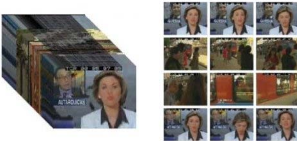
12 13 14 15 16 17 18 19 20 21 22 23 24 25 26 27 28 29 30 31 Fig. 2 Video Streamer and VideoIndex . Video user interface techniques that show the structure of the 32 video. The images in the index are chosen with image processing algorithms for shot detection.
